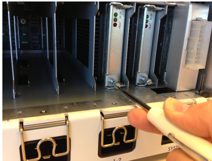
Figure 8. Secure the Bracket with Slotted Screwdriver
