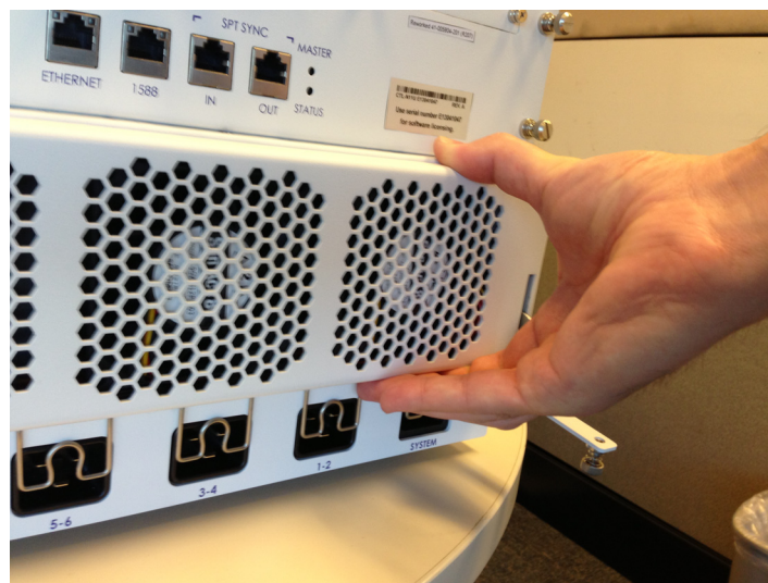
Figure 3. Gently Rock Fan Tray Panel to Remove
