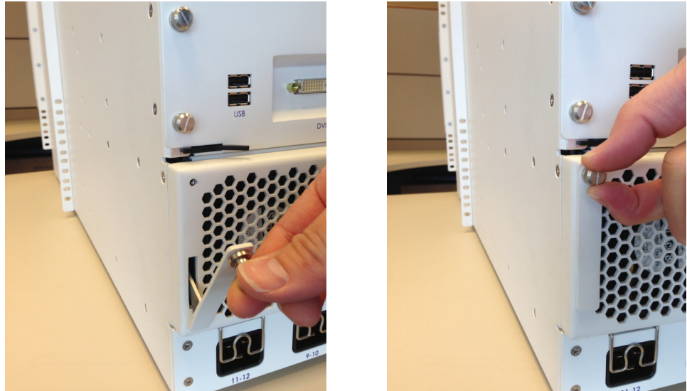
Figure 10. Fold up the Brackets and Tighten Thumbscrews
