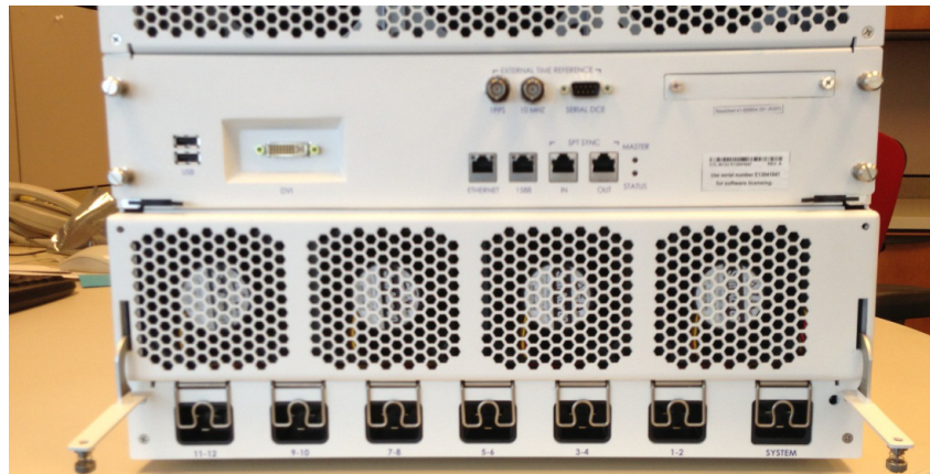
Figure 9. Fan Tray in Place with Brackets in Unsecured Position
