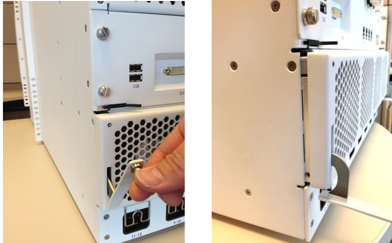
Figure 2. Pull Down the Latches
